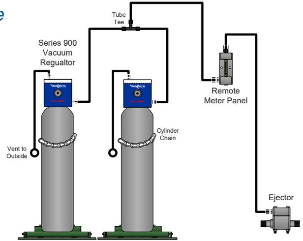
Hydro Instruments Series 900 Gas Chlorination System with Integral Switchover
